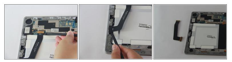
• Using the black nylon spudger, for the black ribbon cable you must gently apply pressure up from underneath until you hear a popping sound.
