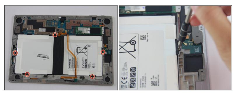
• Using a J000 screwdriver, unscrew the five 3.4 mm Philips screws.
