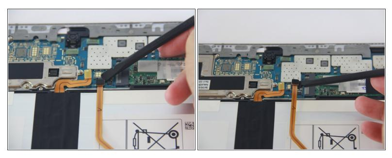
Use the black nylon spudger tool to gently remove the long orange ribbon cable from the motherboard.
