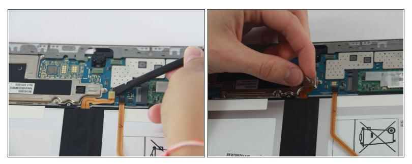
Use the black nylon spudger tool to gently remove the small orange ribbon cable from the motherboard.
