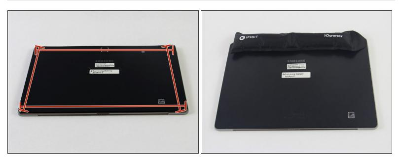
Heat the iOpener in the microwave for 30 seconds. Then place it on each side for 20 seconds in order to loosen the adhesive sealing on the device.
