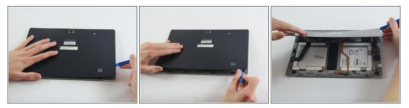
• Using the plastic opening tool, open up the back of the device.
