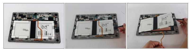
• After removing the leftmost ribbon cable and all five screws, we can then use a black nylon spudger to lift the battery out of the device.
