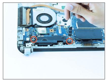
Remove the two 7mm screws with a Phillips #0 screwdriver.
