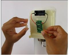
Wedge the plastic spudger between the microchip and the glue dot until the glue pops off.
