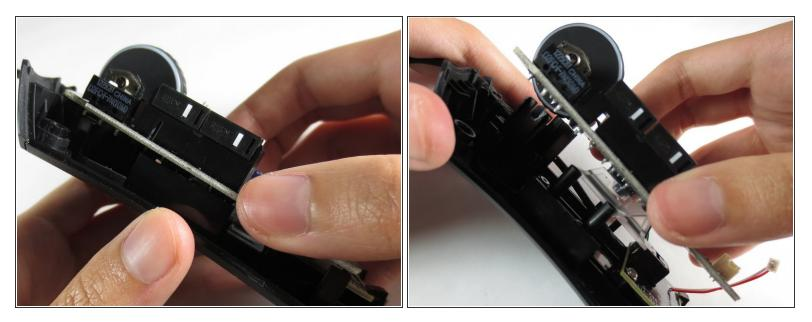
• Remove the motherboard by grasping the sides and gently pulling upward.
