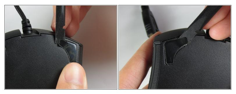
• Use the blunt end of the spudger to pry the adhesive rubber pads from the top left and right edges.
