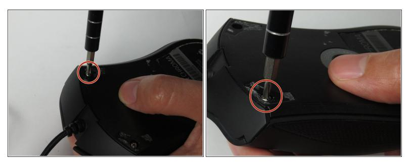
Use a Phillips #0 screwdriver to remove two 6.7 mm screws.
