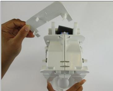
Unhook the four clips on the top of the carbonating block and remove the plastic cover.
