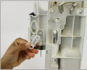
Remove the plastic piece, located near the front of the carbonating block, from both sides of the device using a plastic opening tool or nylon spudger.
