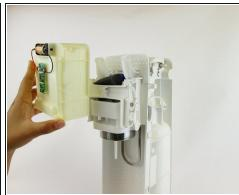
Slide the yellow battery cover up and away to remove it from the device.
