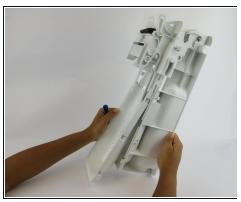
Lift the clips located on both sides with the plastic spudger. Slide the front cover off.
