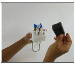
• Pull the foam pad up and remove it from the front side of the carbonation component.
