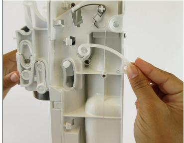
• Lift the top of the plastic arm with the spudger and remove it on both sides.
