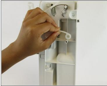
• Unhook the bottom piece of the plastic arm on each side of the device.
