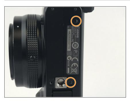
After removing the first screw flip to the bottom side of the camera and unscrew the two screws located toward the back side of the casing. The screw on the front side can be left in. Use a Phillips Head 00 screwdriver for both of these screws.
