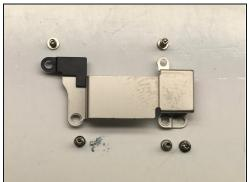
• Remove the five screws holding the earpiece speaker retaining plate in place. These are #000 phillips head screws.
