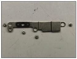
• Using your #000 tri-tip screwdriver remove the four screws holding the home button backplate in place.
