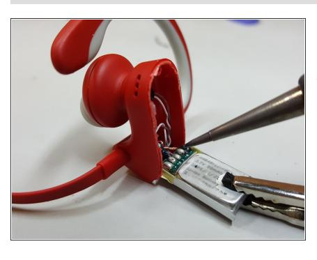
Desolder battery using soldering iron and replace with replacement battery.
