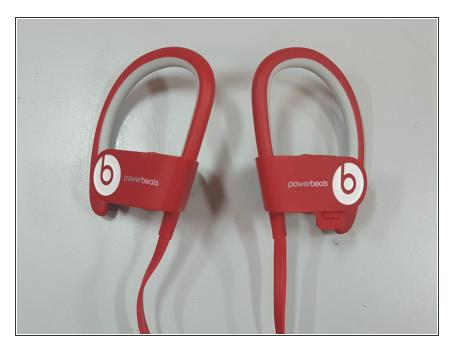
The battery is located inside the right side ear piece.
