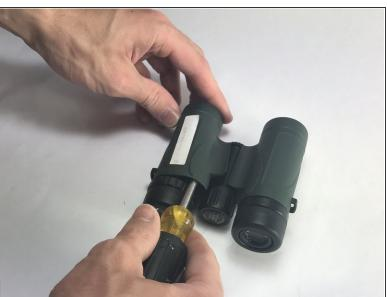
Using a plastic opening tool, nylon spudger or metal spudger, pry into seam of the skin cover at the center of the device. Lightly lift the tool which should cause the skin cover to rise.
