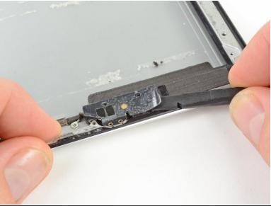
Use the flat end of a spudger to loosen the foam adhesive holding the Wi-FI antenna to the speaker assembly.
