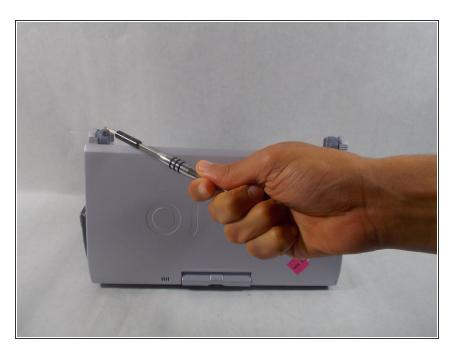
Remove the 6 mm Phillips #0 screw on the left side of the battery that holds the casing to the device.
