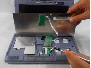
• Lift up underneath the keyboard using the iFixit opening tool to expose the ribbon wires connecting the keyboard to the motherboard.
