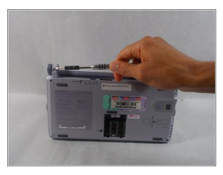
Turn the device upside down and remove the 6 mm Phillips #0 screw holding the casing to the device.
