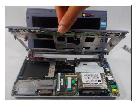
Remove the top casing by lifting up on the plastic exposing the two speakers.
