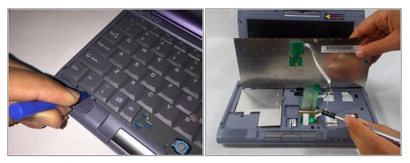
Lift up underneath the keyboard using the iFixit opening tool to expose the ribbon wires connecting the keyboard to the motherboard.
