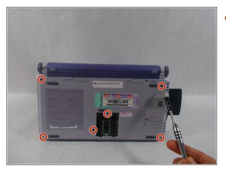
Turn your device upside down and remove the 6 10mm screws attaching the back casing to the device using a phillips head screwdriver.
