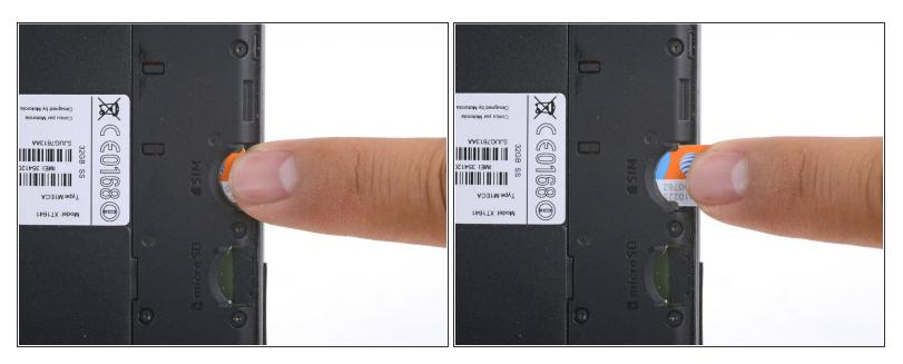
Slide out and remove the SIM card.
