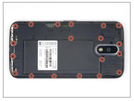
Remove the nineteen 3.1 mm T3 screws securing the midframe.
