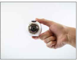
Twist silver ring on the lens counter-clockwise with force to remove it.
