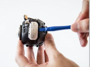
Carefully use a plastic opening tool to separate the gray case from the black case on the device.
