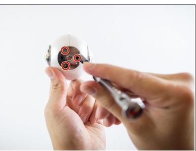
Once the black rubber has been removed, unscrew all Phillips #00 0.75 mm screws on the bottom of the device using a PH00 screwdriver head.
