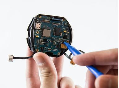
Use a plastic opening tool to disconnect the sensors from the motherboard to free it.
