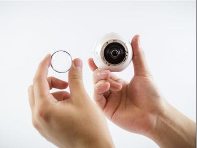
Insert a small flathead screwdriver into marked slot on camera lens and pry off camera lens cover.
