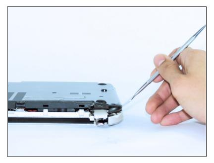
• Run the spudger or a <u>plastic</u> <u>card</u> around the entire laptop to release the rest of the clips.
