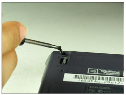
Use the Phillips #00 screwdriver to remove the two screws near the top of the device.
