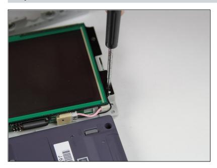
Use the Philips #00 screwdriver to remove the three screws in the corners of the screen.
