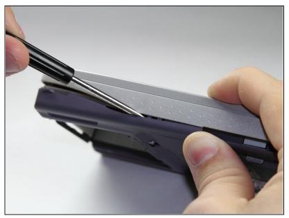
Use a spudger or opening tool to separate the two halves of the case.
