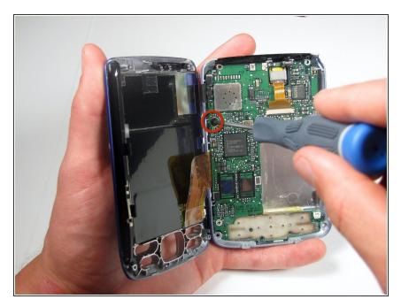
Unscrew the single 3.5mm screw attaching the motherboard to the case with a #00 Phillips screwdriver.
