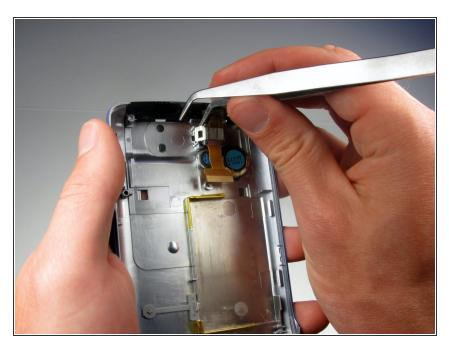
Using tweezers, pry one side of the clip off.
