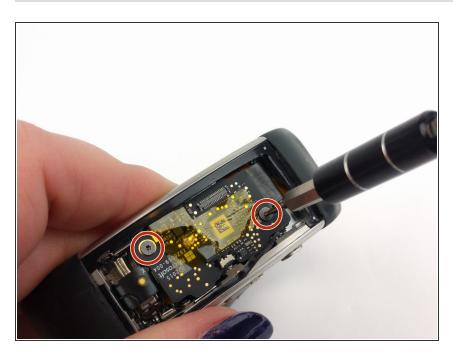
Use the T3 Torx Screwdriver to remove the two 2.7 mm screws
