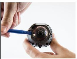
Carefully lift the three sensors off using a plastic opening tool and pull them aside.
