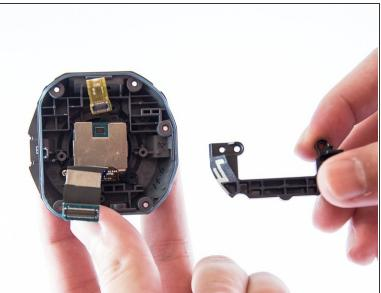
Using a plastic opening tool, remove the plastic cover underneath the rear camera
