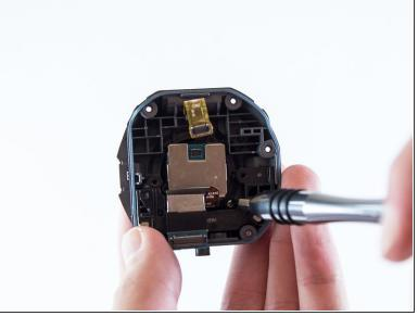
Using a PH000 screwdriver head, remove the both Phillips #000 0.75 mm screws on the grey case.
