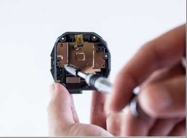
Within the grey half of the case, unscrew both Phillips #00 0.75 mm screws located on the metal plate using PH00 screwdriver.
