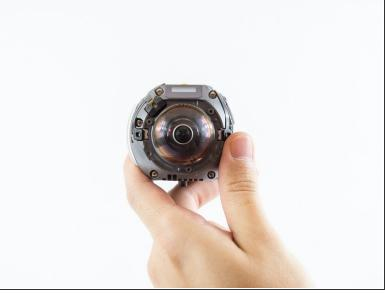
Remove all Phillips #00 0.75 mm screws from the body of the camera using a PH00 screwdriver head.
