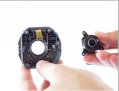
Gently remove the rear camera module by using a plastic opening tool and lifting the module.
