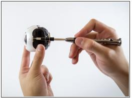
• To remove the left cover of the camera body, lift the left cover using a small flathead screwdriver and pull it off.
