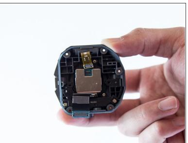
Once the screws have been removed, remove the metal plate.
