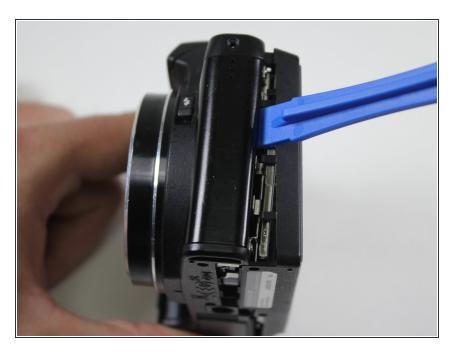
Using the blue plastic opening tool, wedge open and remove the case.
