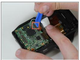
Lift the retaining flaps on the three remaining ZIF connectors connected to the motherboard.
