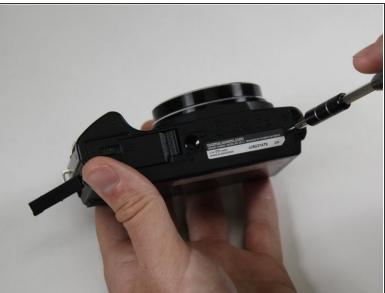
Remove nine 4.45mm Phillips #000 screws from the outside of the case.
