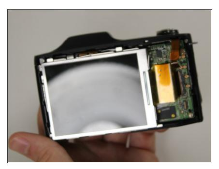
Once you have the back case off, remove the LCD Screen.
