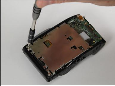
Remove the four 3.8mm Phillips #000 screws from the LCD frame.
