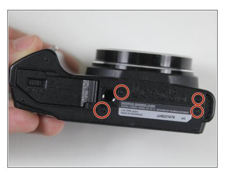
There are four screws to take out on the bottom of the camera.
