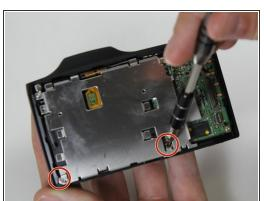
Remove the top left screw, top right screw, bottom left screw, and bottom right screw from LCD frame.
