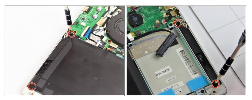
• Unscrew the two 6.5mm screws from each speaker with a PH1 Phillips head screwdriver.
