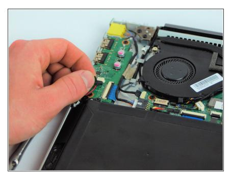
Disconnect the speaker cable connectors from the motherboard and/or USB board.
