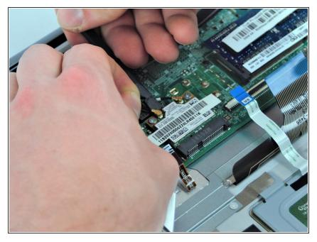
• Use the plastic spudger to lift and disconnect the antennae connectors from the motherboard.
