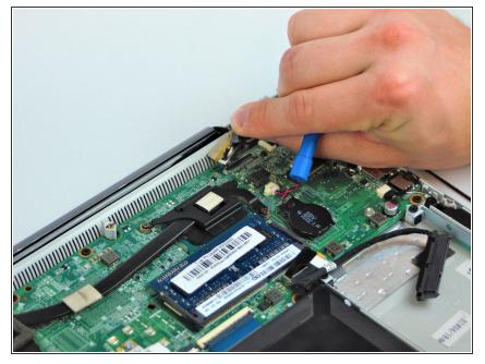
Use the plastic opening tool or spudger to lift and remove the flat top connector from the motherboard.
