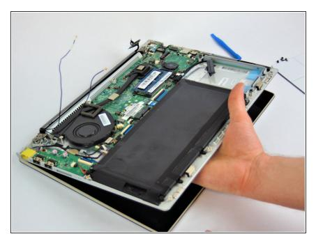
• Carefully separate the bottom of the laptop from the screen.
