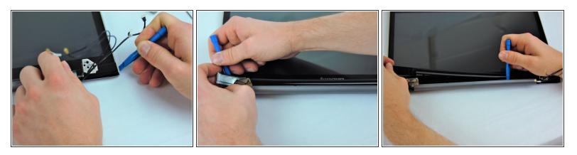
• Using the spudger and the plastic opening tool, carefully remove the plastic cover from the bottom of the screen.
