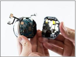
Insert a plastic removal tool underneath the four sensors on the motherboard to fully separate the camera case.
