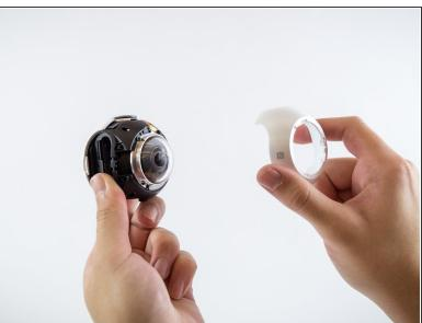
Using both hands, carefully remove the right cover off the camera body.
