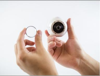
• Insert a small flathead screwdriver into marked slot on camera lens and pry off camera lens cover.
