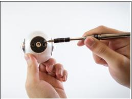
Peel off the black rubber located on the bottom of the device using your hand or a small flathead screwdriver.
