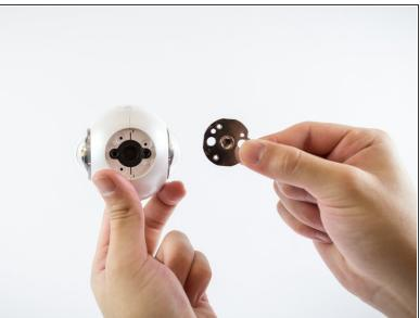
Using a plastic opening tool, pry the tripod mount off the device.
