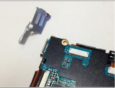
Remove the copper phillips screw holding the HDMI mounting plate and detach the mounting plate.
