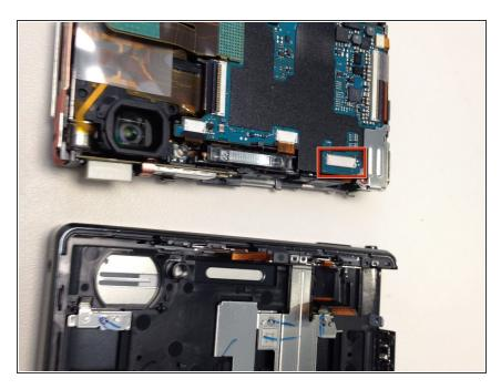
Gently pull and disconnect the ribbon cable connecting the front cover to the main body
