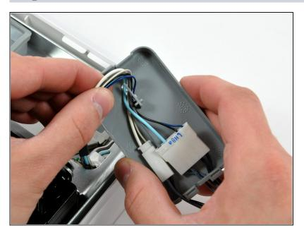
• De-route the inverter cables from the inverter cable cover hook.
