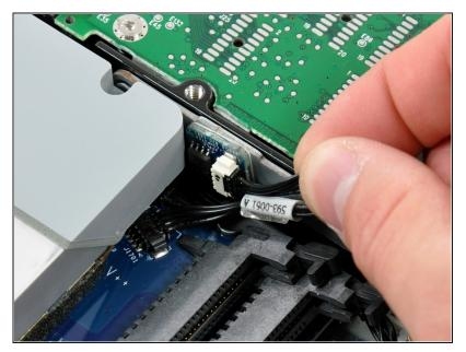
• Disconnect the hard drive thermal sensor cable from the thermal sensor board on the hard drive bracket by pulling the cable away from the heat sink.
