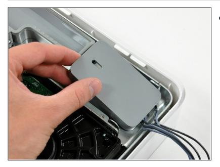
• Flip up the inverter cable cover from its left edge and lift it out of the chassis.
