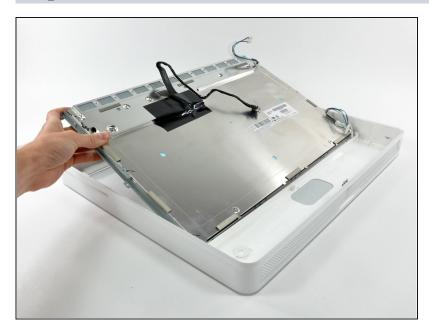
• Lift the display out of the front case.
