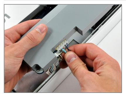
• Disconnect the large inverter cable connector from the inverter by pulling straight away from its socket.
