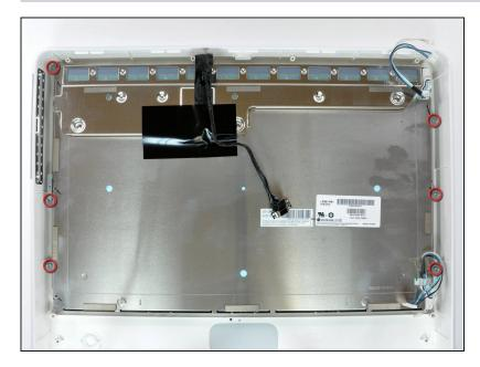
Remove the six 7.2 mm coarsethread T10 Torx screws securing the display to the front case.
