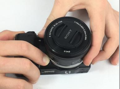
• While holding down the button, twist the lens counter-clockwise until you hear and feel a firm click.
