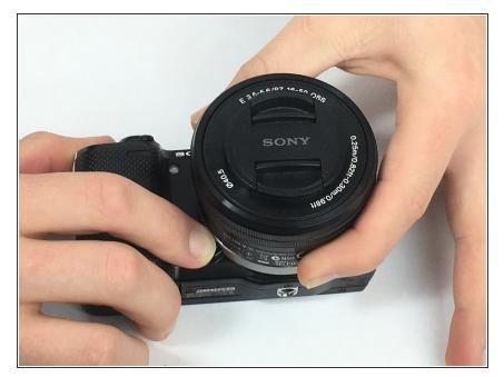
With the camera facing you, push down on the button located to the bottom left of the lens.
