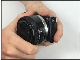
To put the lens back on , line up the white dot on the lens with the white dot on the e-mount. Twist clockwise until you hear and feel a firm click.
