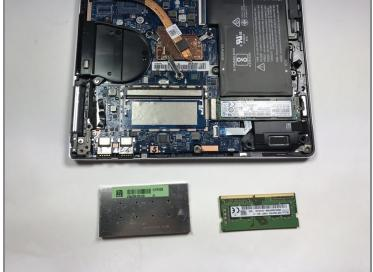
• Remove the RAM by pulling away from the RAM socket.
