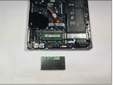
• Use blue plastic opening tool to pry the ram cover loose. Carefully lift up the ram cover and remove it from the laptop.
