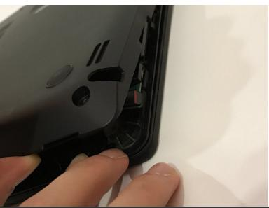
After removing all of the screws, gently lift up on all covers to remove the back plate and reveal the interior of the device.
