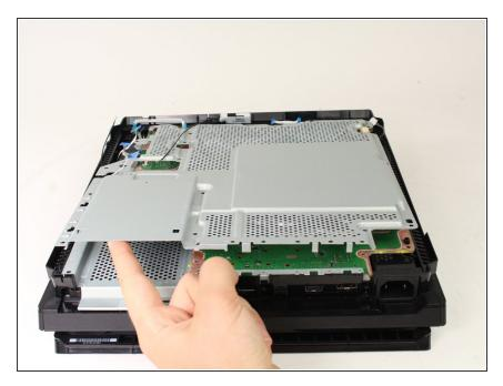
Pull up and remove the metal plate.
