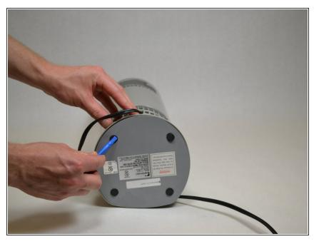
Using the plastic opening tool, turn the device over and remove the black plastic covers over the four screw holes.
