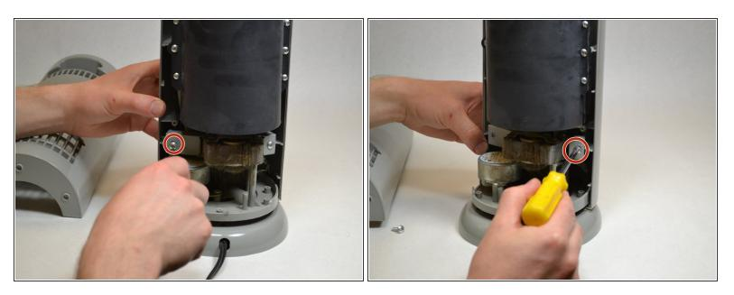
• Remove the 2 screws that attach the front part of the casing to the motor.
