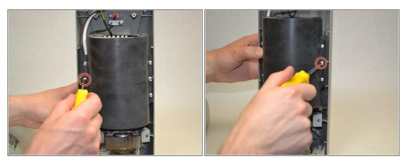
Remove the two middle screws attaching the black plastic cover to the front.
