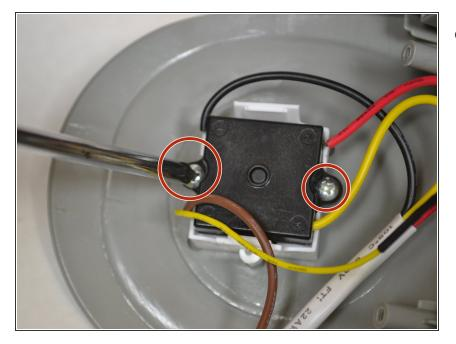
Remove the two screws keeping the button attached to the top of the casing.
