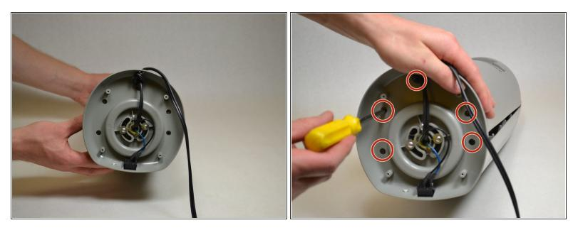
• Remove 5 smaller screws visible through small holes between the base and the casing.
