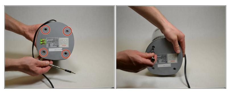
Remove the four screws underneath the plastic covers.
