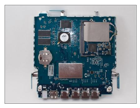
Take the device out of the casing and orient it so that you can see the WiFi card.
