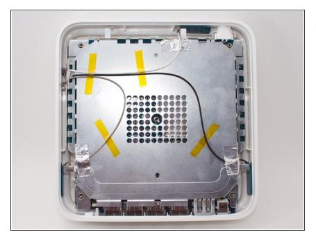
After unscrewing all five screws, remove the plastic casing. The back should now look like the picture shown.
