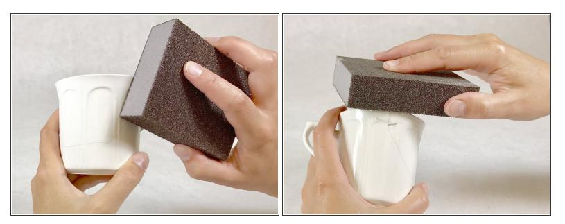
• Use coarse sandpaper to further reduce the excess epoxy.
