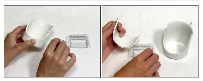
Apply the epoxy along the edges of the base piece of china and first chipped piece of china using the toothpick.
