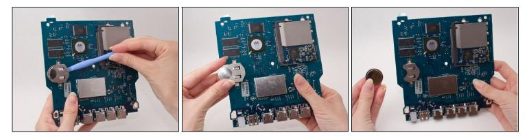
• Remove the battery by gently "shoving" it out with the plastic tool.
