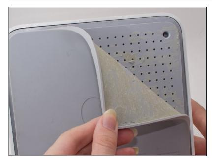
• First start by peeling off the outer rubbery covering on the bottom of the device.
