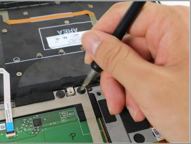
Remove the four 3 mm Phillips #1 screws from the trackpad.
