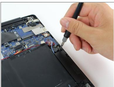
Remove the four 3 mm Phillips #0 screws located on each corner of the battery.
