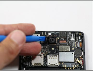
Disconnect the rear-facing camera from the motherboard by pulling out the press-fit connector to its left.
