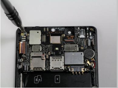
Remove the two 2.9mm Philips #00 screws.
