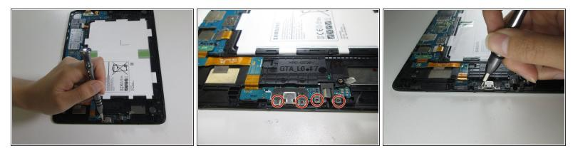
Remove the four 2.8mm #000 Phillips screws that hold the charging port and headphone jack in place.
