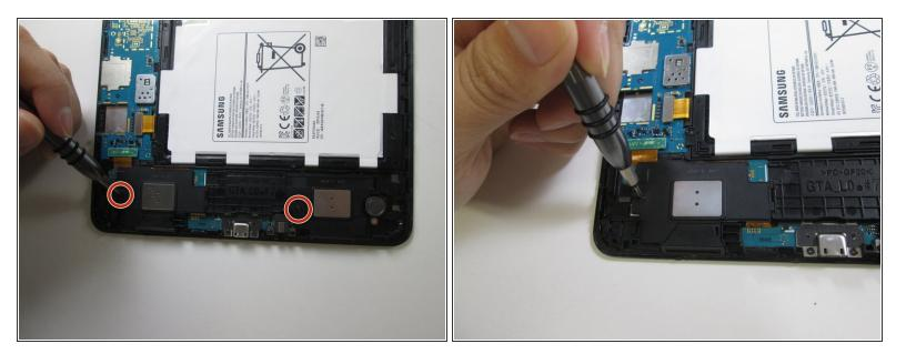
Remove the two 2.8 mm Phillips #000 screws from the speakers.
