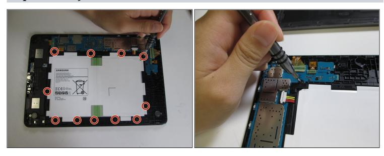
• Remove the eleven #000 Phillips 2.8mm screws that hold the battery in place.
