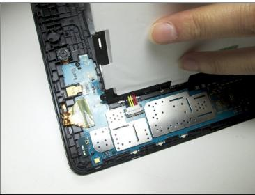
• Pull the battery out until it is only connected to the device by the black, yellow, and red connectors.
