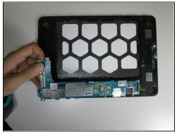
• Using your fingers or a spudger, gently remove the motherboard from the device.
