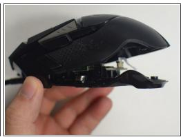
Use a nylon spudger to pry the top shell from the bottom of the mouse.
