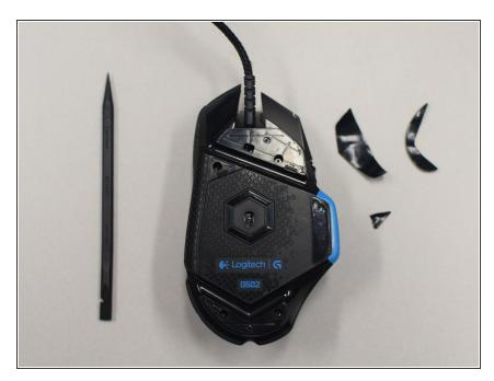
Use your fingers or a nylon spudger to remove the specified mouse feet in order to reveal the screws.
