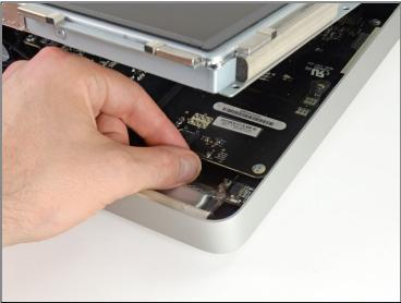
Using your fingers, carefully pull the vertical sync cable out of its socket on the LED driver board near the top left corner of your iMac.
