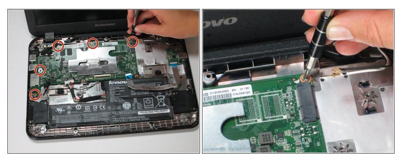
• Use a screwdriver to remove the five 3.0mm Phillips screws from the motherboard.
