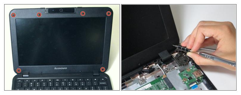
• Remove the six 4.0mm Phillips screws that are underneath the rubber pads with a screwdriver.
