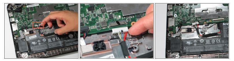
• Disconnect the battery by pulling the battery cable connector straight out.
