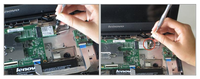
• Use a screwdriver to remove the single 3mm Phillips screw that is holding the WiFi card in place.
