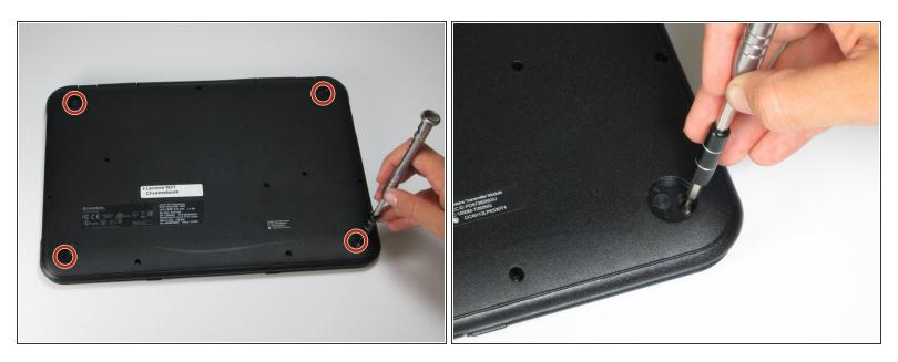
Use a screwdriver to remove the four 5.0mm Phillips screws located under the rubber soles.
