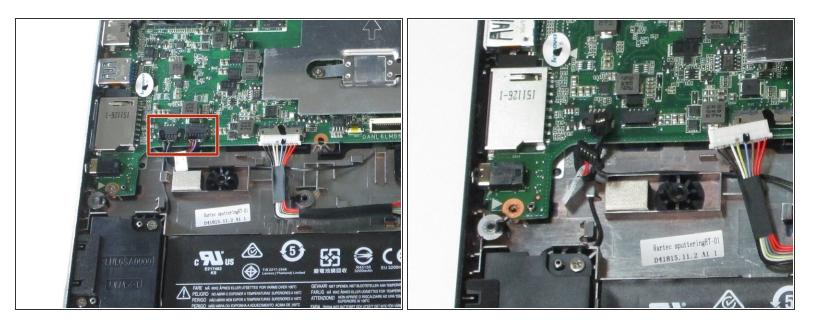
Disconnect the speakers by pulling the two speaker cables straight out of their connectors.
