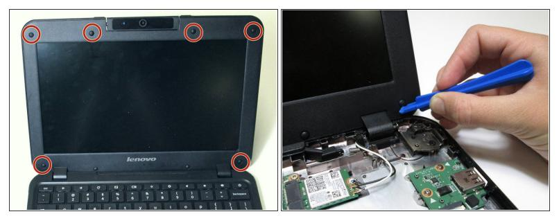
Carefully pry off the six small rubber pads around the screen with a plastic opening tool to expose the screws.
