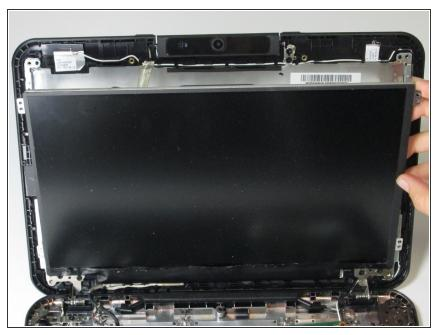
• Remove the screen from the device.
