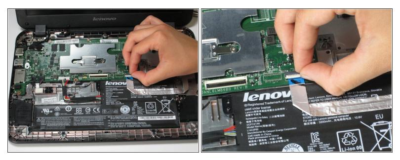
Disconnect the USB cable from its ZIF connector by lifting up on the ZIF tab and pulling the cable straight out.
