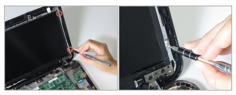
• Remove the four 3.0mm Phillips screws symmetrically placed on either side of the screen.
