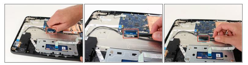
Lift the black clasp and use the spudger tool to remove the ribbon so that it completely disconnects from the motherboard.
