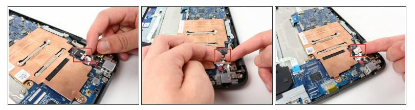
Locate and gently pull the wire harness (small plastic box with two pink, one orange, and two black wires) directly out of the connector on the motherboard.
