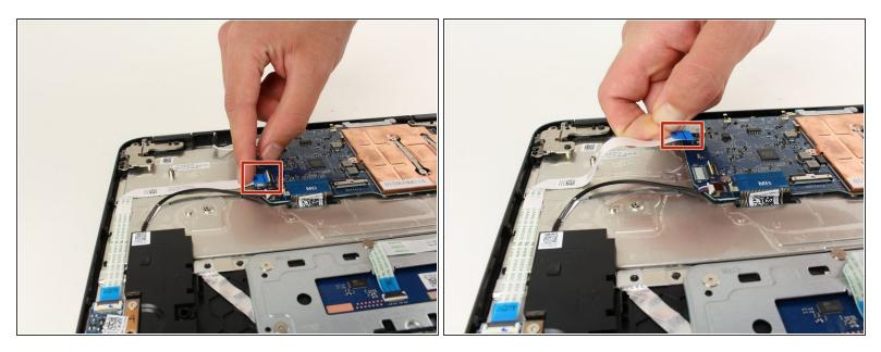
Lift the black clasp and gently pull on blue ribbon until it completely disconnects from the motherboard.
