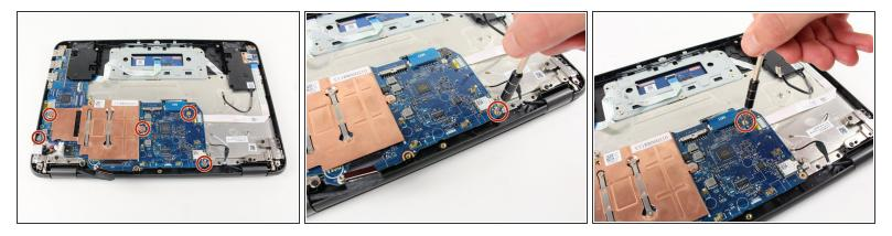
• Using a Phillips #0 screwdriver, remove the five 3mm screws.
