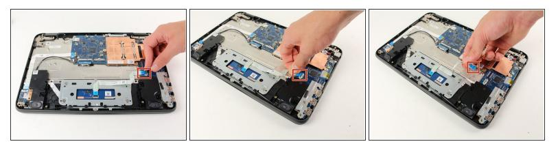
Lift the black clasp and gently pull on blue ribbon until it completely disconnects from the motherboard.
