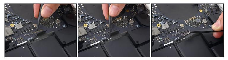
• Use the tip of a spudger to flip up the retaining flap on the keyboard data cable ZIF socket.
