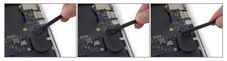
Use the flat end of a spudger to pry the left speaker connector up and out of its socket on the logic board.
