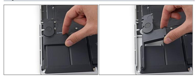
• Remove the right speaker by pulling it slightly away from the side of the upper case, and out from under the aluminum tab blocking it in.
