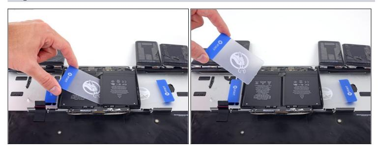
• Remove the first card that you inserted under the final battery cell.
