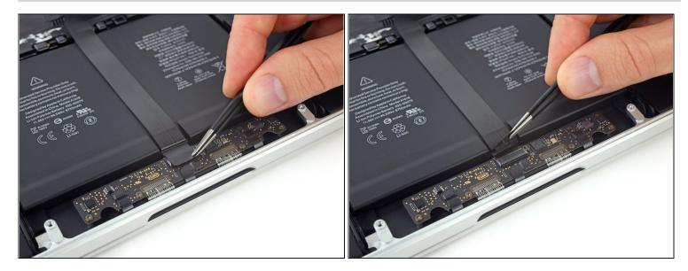
• Peel back the tape covering the trackpad connector ribbon cable, near the front edge of the MacBook Pro.
