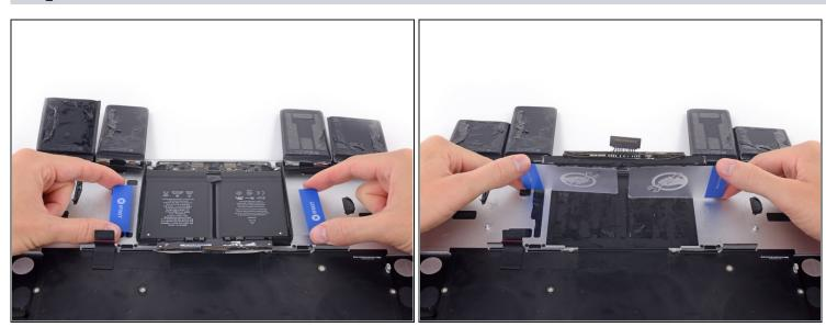
• With one plastic card underneath each of the two center battery cells, twist and lift both cards to fully separate the battery cells, together with the plastic frame and battery board, from the MacBook Pro.
