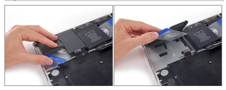
• Flip the two de-adhered right-hand battery cells over the front edge of the MacBook Pro, if you haven't already. This will allow access to the outside edge of the center cell.
