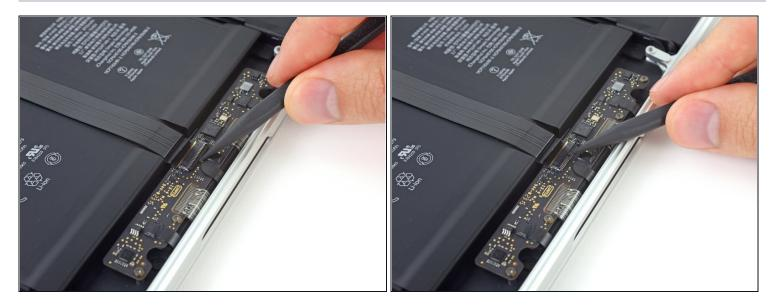
Use the tip of a spudger to flip up the black locking tab on the trackpad ribbon cable ZIF connector.
