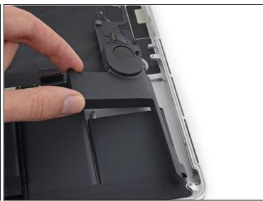
Remove the left speaker by pulling it slightly away from the side of the upper case, and out from under the aluminum tab blocking it in.
