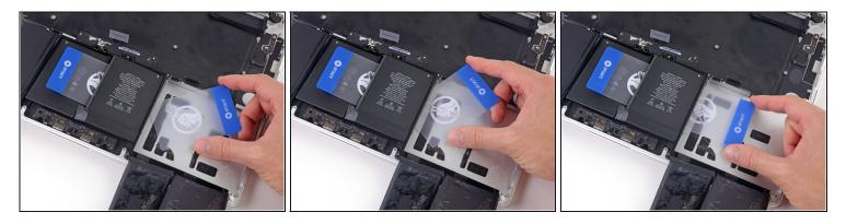
• Push one corner of a plastic card below the plastic battery frame and underneath the remaining adhered edge of the lower center cell.
