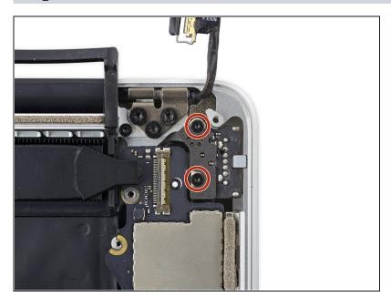
Remove the two 4.0 mm T5Torx screws from the MagSafe 2 board.
