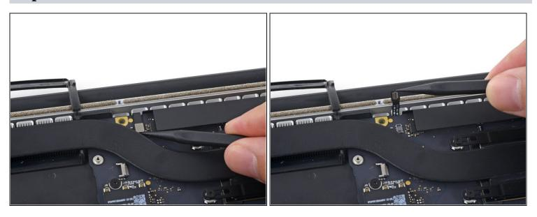
Use the point of a spudger to pry the keyboard backlight connector up from its socket on the logic board.
