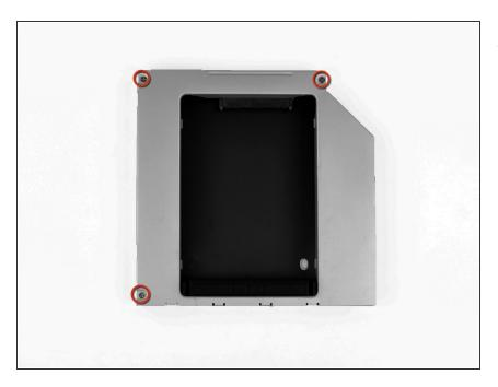
Remove the three 3.0 mm Phillips screws from the optical bay enclosure.
