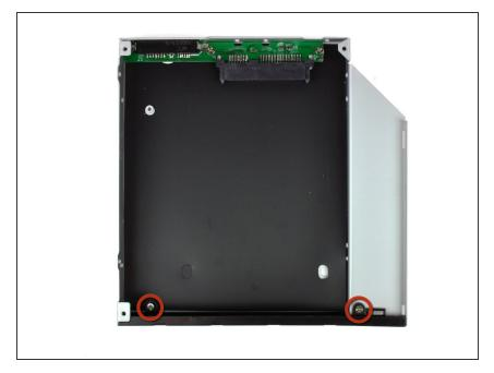
Remove the two 3.0 mm Phillips screws securing the faceplate to the optical bay enclosure.
