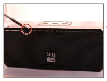
• Pull out the two black wire meshes using a metal spudger.
