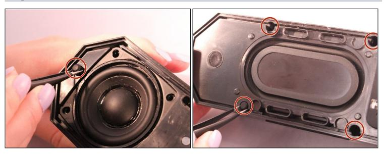
• Using <u>tweezers</u> remove the rubber stoppers (4 at the back + 2 at the front).
