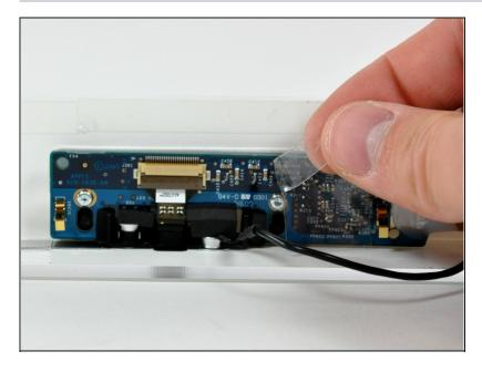
• Remove the strip of tape covering the camera board.
