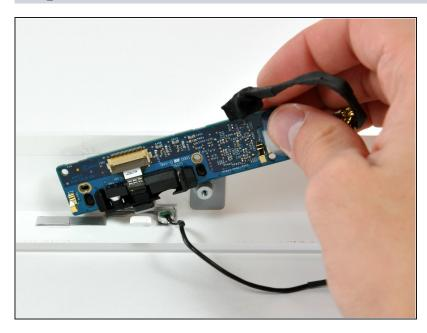
• Lift the camera board out of the front bezel.
