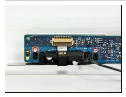
• Remove the two T6 Torx screws securing the camera board to the front bezel.
