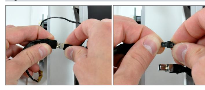
Disconnect both the camera and microphone cables.
