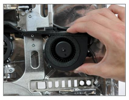
Pull the optical drive fan off the posts protruding from the rear case and lift it out of rear case, de-routing cables as necessary.
