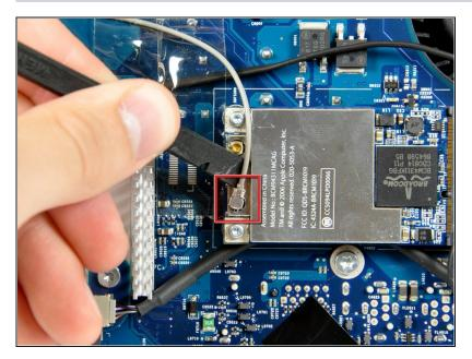
Use the flat end of a spudger to pry the AirPort Extreme antenna connector up off the AirPort Extreme card.
