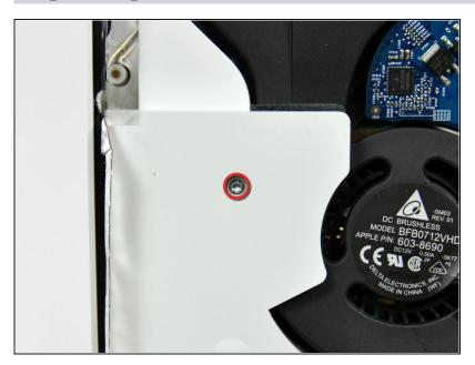
Remove the 30 mm T10 Torx screw securing the left speaker to the rear case.
