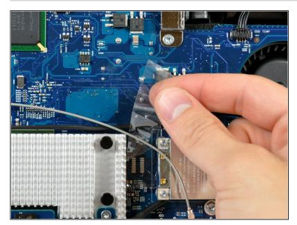
*i* If necessary, remove any tape covering the left speaker cable.
