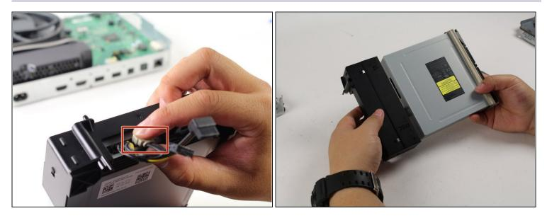
• Detach the wires from the disc drive and slide the drive out.
