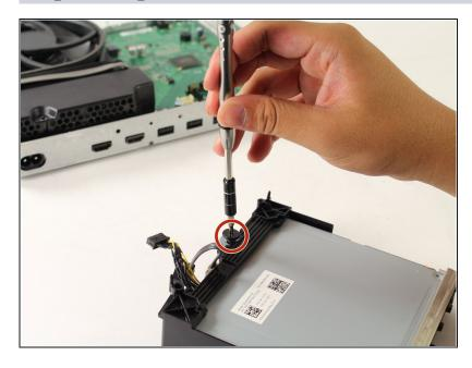
• Remove the black, flat Torx screw from the bottom of the optical drive.
