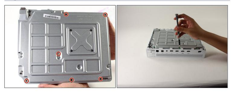
• Use a T10 Torx screwdriver to remove the six green 50 mm long screws from the metal case labeled F1 through F6.
