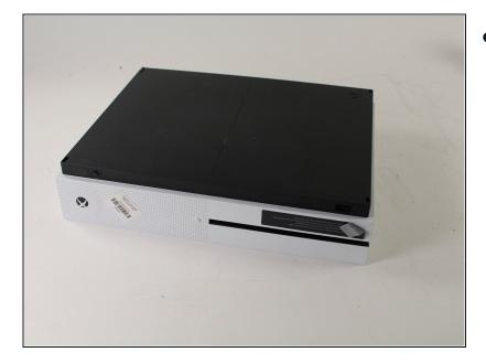
Flip the Xbox One S so that the bottom of the case is facing upward.
