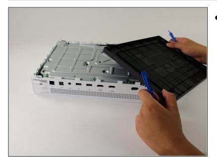
• Once all of the clips are opened, remove the bottom part of the case.
