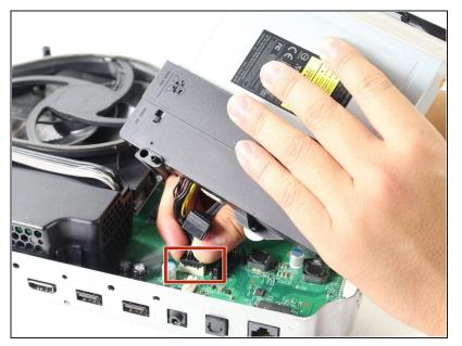
Pull the disc drive slightly off the motherboard and disconnect the plastic connectors from the motherboard.
