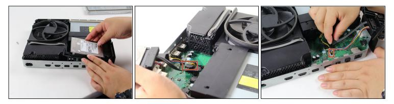
Gently disconnect the hard drive from the motherboard (at the two plastic connector bodies).
