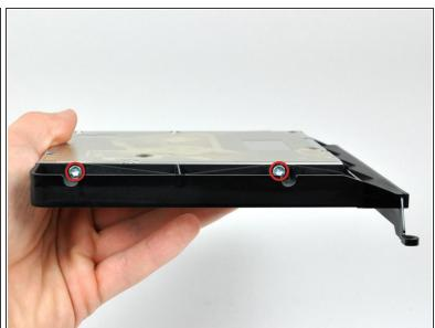
Remove the two T10 Torx screws from both sides of the optical drive (four screws total).
