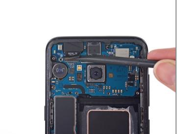
• Use the flat end of a spudger to disconnect the front-facing camera connector.
