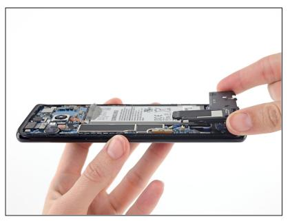
Remove the loudspeaker assembly.
