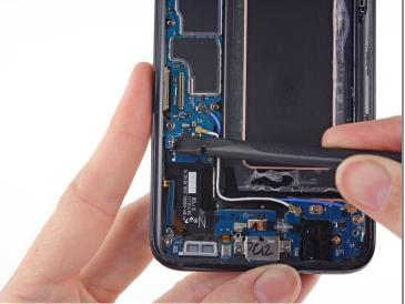
Use the flat end of a spudger to disconnect an antenna ribbon cable that connects the motherboard to the daughterboard.
