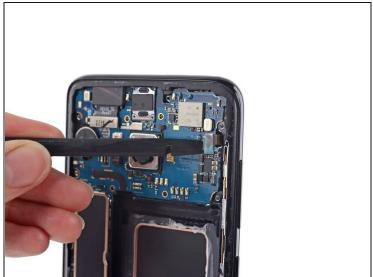
Use the flat end of a spudger to disconnect the sensor array connector.
