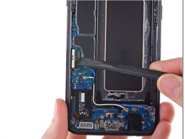
Use the flat end of a spudger to disconnect the display and digitizer connector.
