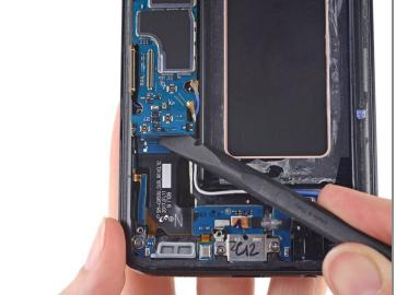
Use the flat end of a spudger to lift the motherboard and disconnect it from the daughterboard.
