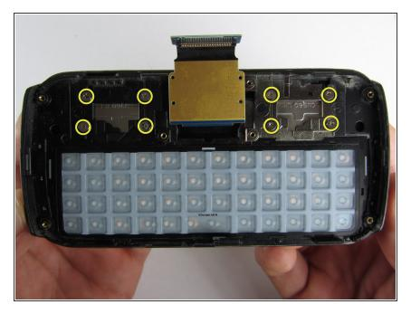
Remove the eight 1.7mm Philips screws above the keyboard.
