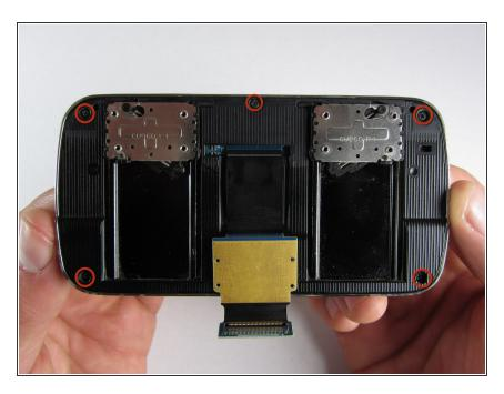
Remove the five 3.0mm Philips screws around the outside of the sliding mechanisms.
