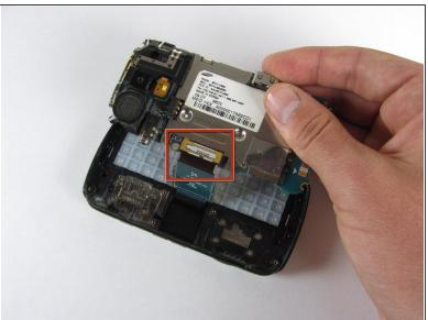
Carefully lift the motherboard up from the bottom edge.
