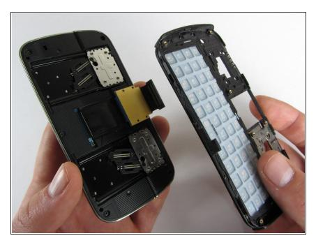
Carefully remove keyboard frame from the sliding mechanisms underneath.
